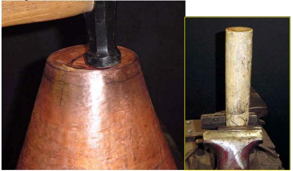
As the vessel is being raised the stake should be resting against the bottom of the vessel. This will cause the bottom to bulge out and become irregular. Setting the bottom again straight will help keep the vessel true and at the designed diameter.
