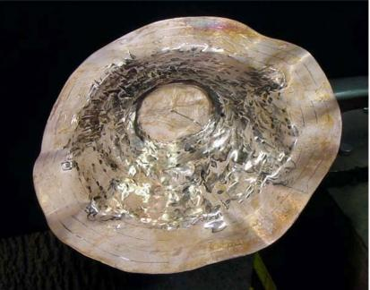
The first round on the disc looks pretty ugly and all ruffle. About 2/3 of the rows have been completed. You can see the disc is folding as it is being raised, which is normal. The important things to remember:
