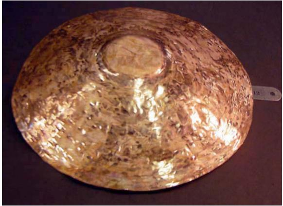
Here is the disc after completing the first round. All of the folds have been closed. The disc is now only 111/2 inch diameter and the sides have been raised about 2 inches. Off to anneal and do some more rounds.
