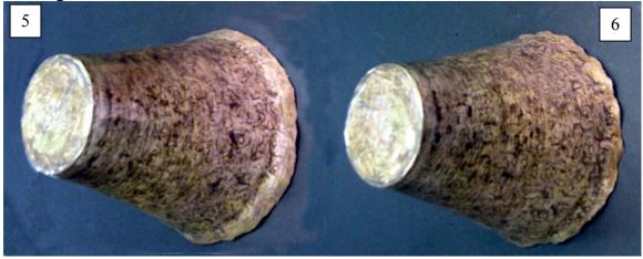
5 – Only two rows to go. Notice how the top diameter is wavy. This is from the metal folding as it is being raised. The folds will be less as the vessel gets smaller in diameter.
