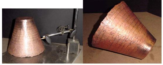
I am a big believer in marking the vessels with the rows and the start lines. Using a compass will only allow you to go so far down the vessel. Here I am using a cheapy magnetic base dial indicator and a steel plate. It may be a little time consuming to do the rows but if you want a vessel to stay true and round it is a must.
