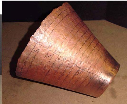
I am a big believer in marking the vessels with the rows and the start lines. Using a compass will only allow you to go so far down the vessel. Here I am using a cheap magnetic base dial indicator and a steel plate. It may be a little time consuming to do the rows but if you want a vessel to stay true and round it is a must.
