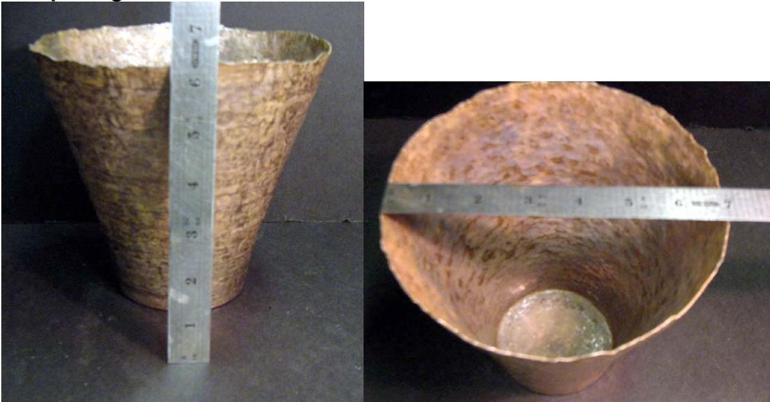
One round of raising is completed. It is not a real fast method. For the time it took to do this one round the size has changed from:
